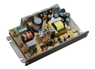
The PSAM65W power supply has dual outputs with power capabilities of 45 watts. With an adjustable +5V out at 3.2A and a +24V out at 1.2A this power supply is efficient to run Anaheim Automation lines of low current microsteppers and programmable controllers. With a compact size of 5.75" x 3.25" x 1.34" and dual mounting position "L Bracket", the PSAM65W can be mounted just about anywhere.
